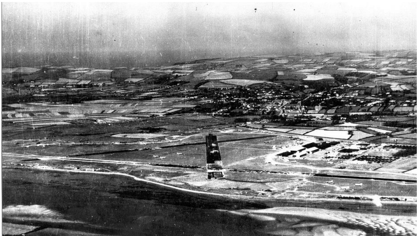
Above – R.A.F. Chivenor taken circa 1944. The photograph is taken from an aircraft probably flying in circuit in an easterly direction parallel with the River Taw (in foreground). Runway 28 – 10 can be seen parallel to the river on its northern bank, with Runway 34 – 16 in the centre. The hangars are to the right of centre, with the wooden huts ('lines') on the right. The railway line can be seen curving alongside the northern perimeter of the base and into the village of Braunton.
