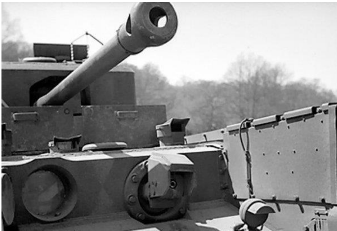
Above – The front of a Churchill Crocodile, showing the nozzle used to discharge the flame from the tank.
