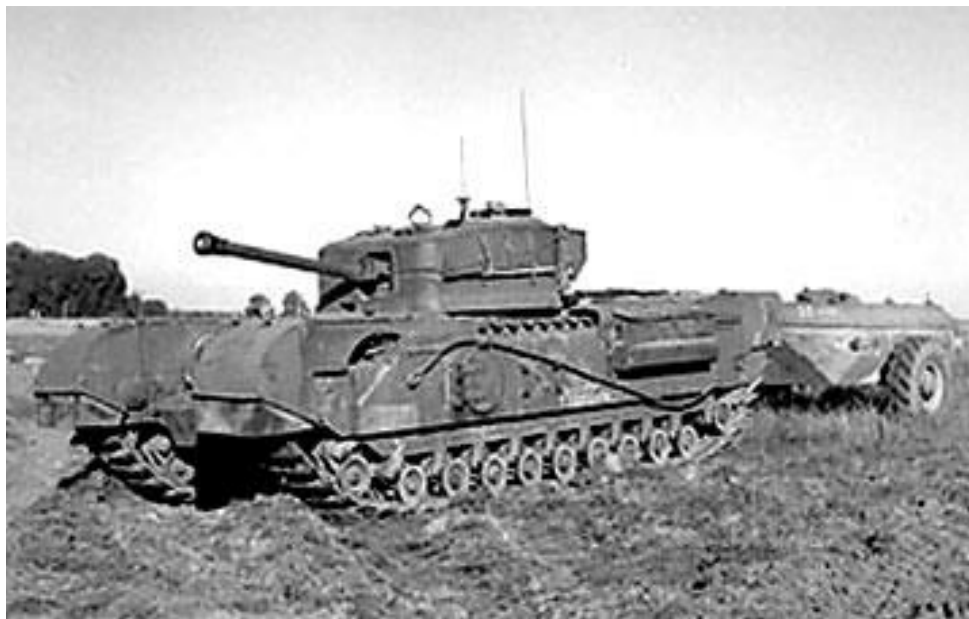
Above – A Churchill Crocodile towing its fuel bowser or trailer.
