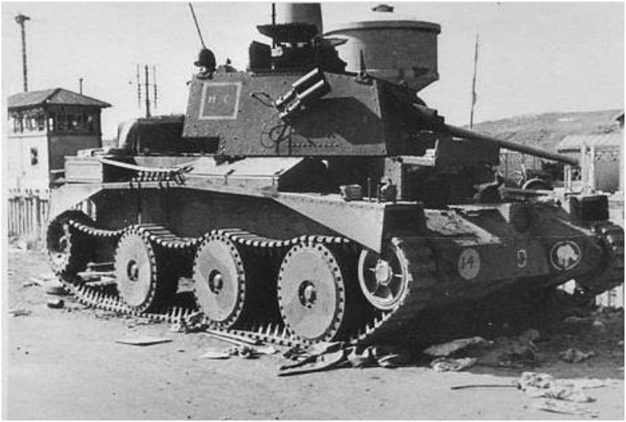
A damaged and abandoned A13 cruiser tank of the 3 rd R.T.R., bearing the white rhinoceros sign of the 1 st Armoured Division. Courtesy of the German Federal Archive.
